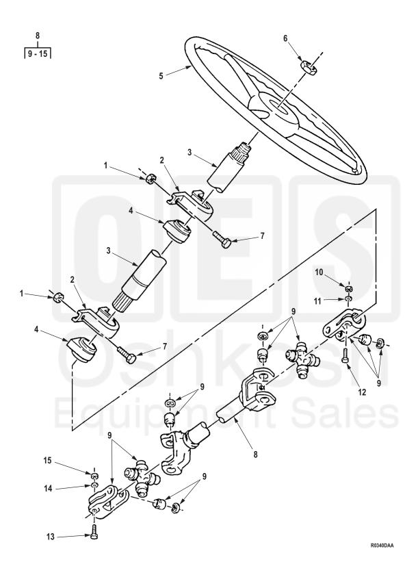
Figure 323. Steering Column, Wheel, and Propeller Shaft.
